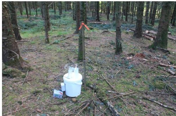
Figure A1. A 6W actinic light set up at a sample plot to survey adult moths.
